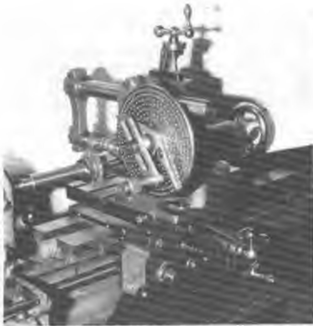
Fig. 56 Showing the Myford Dividing Head fitted onto a vertical slide and mounted on a raising block.
